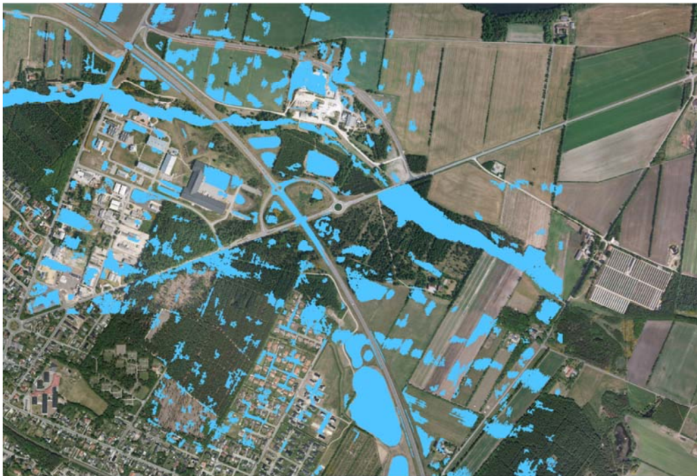
Figure 1. All depressions are identified assuming 100% catchment runoff and no drainage in the depression.
